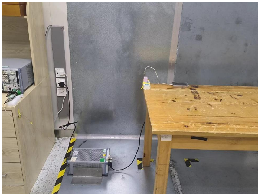
Radiated Spurious Emissions From 30MHz-1000MHz
