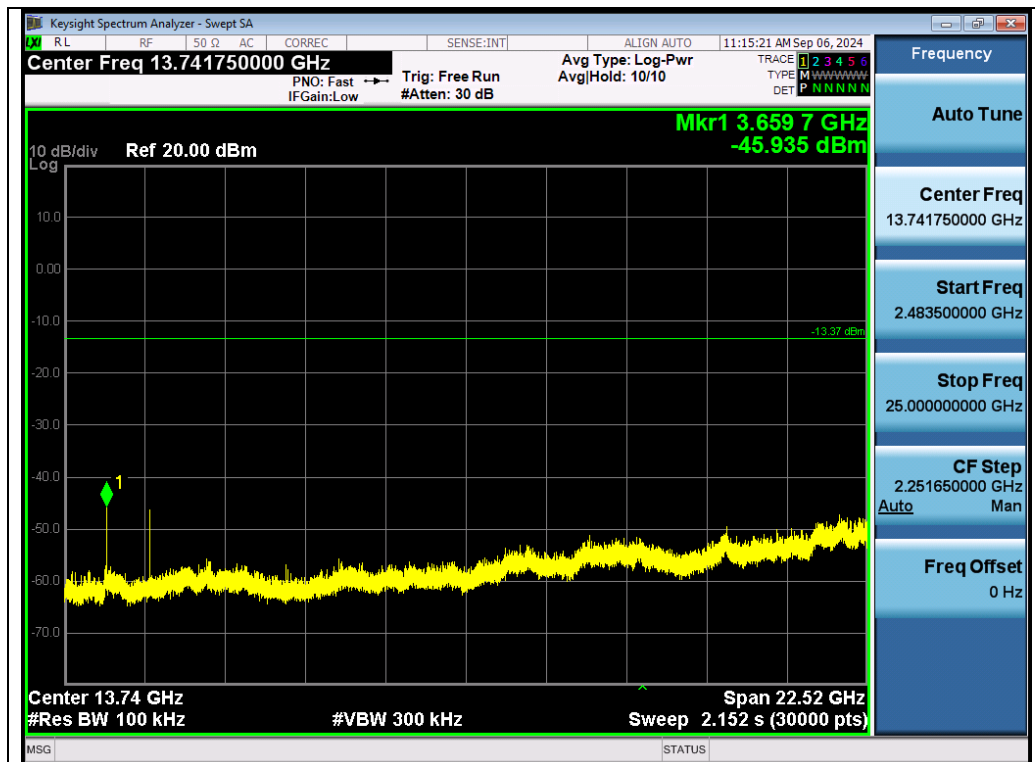
Test_Graph_LE2M_ANT1_2440_2Mbps_Higher Band Emissions
