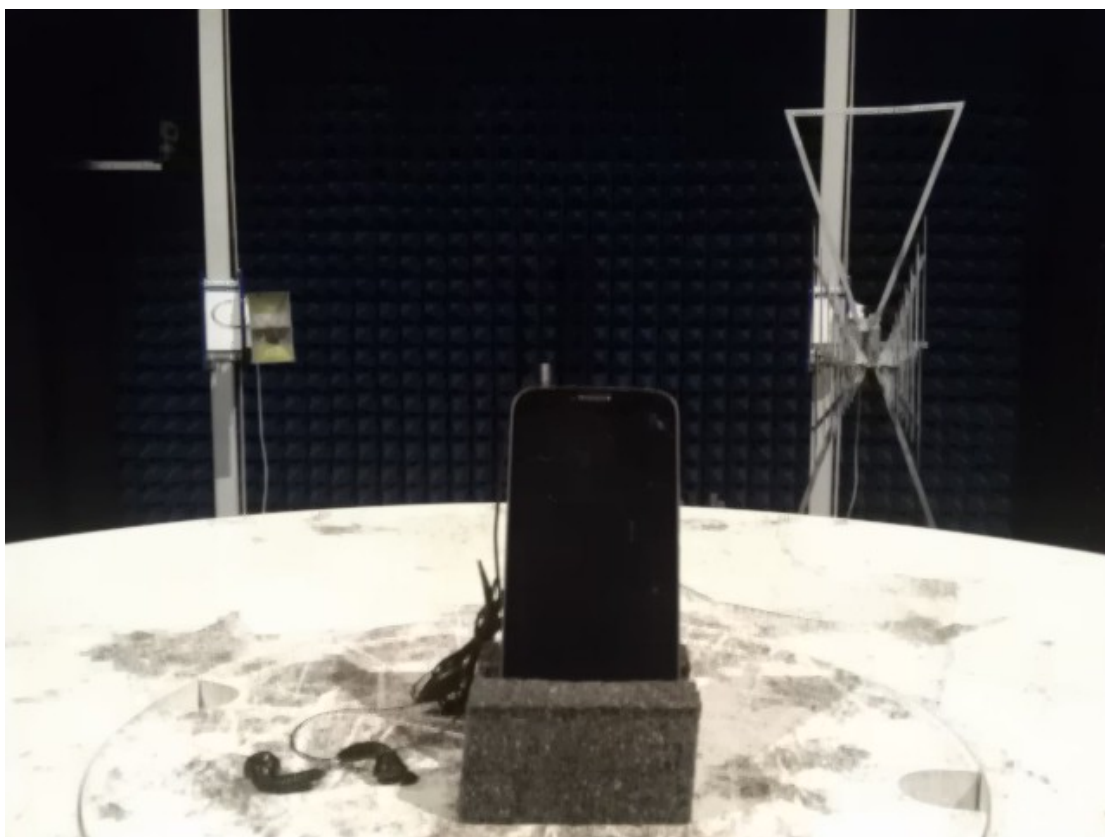
Radiated Spurious Emissions Test setup
