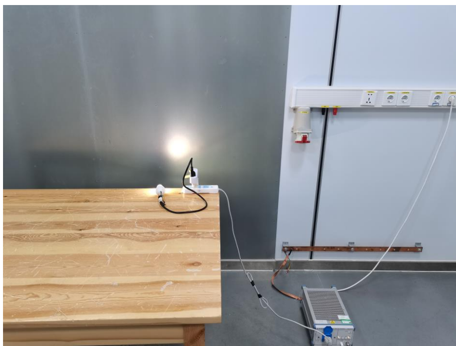
Fig. 4 Power line conducted emission setup photo
