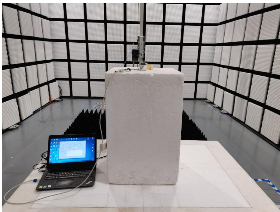
Fig. 3 Radiated emission setup photo(Above 1GHz)
