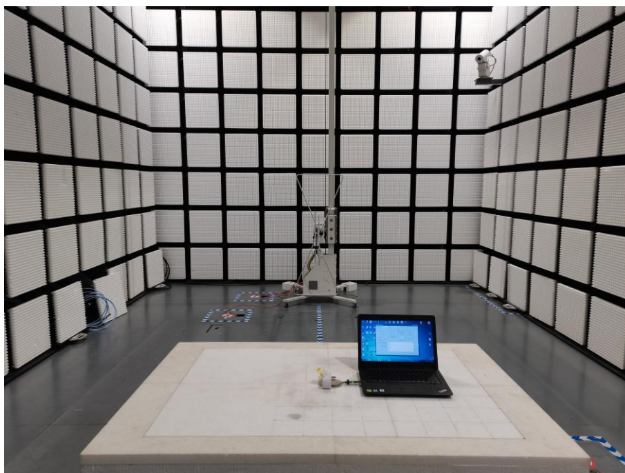
Fig. 2 Radiated emission setup photo(30MHz-1GHz)
