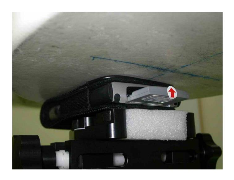
The front of the EUT to the flat phantom distance 14 mm
