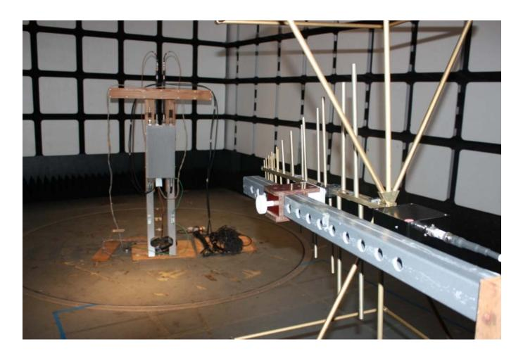
**TEST:** Measurement of Radiated Spurious Emissions
