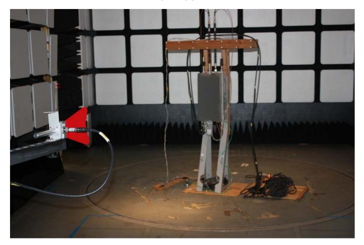
**TEST:** Measurement of Radiated Spurious Emissions
