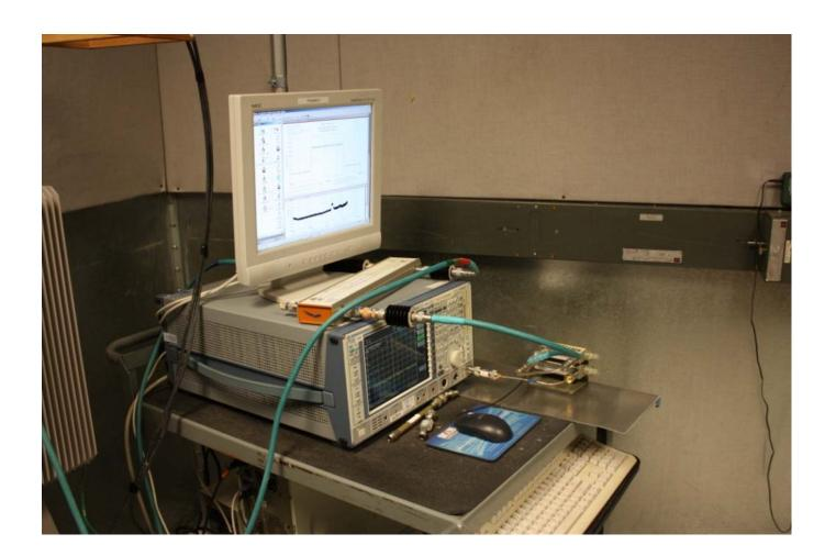
**TEST:** Measurement of Radiated Spurious Emissions
