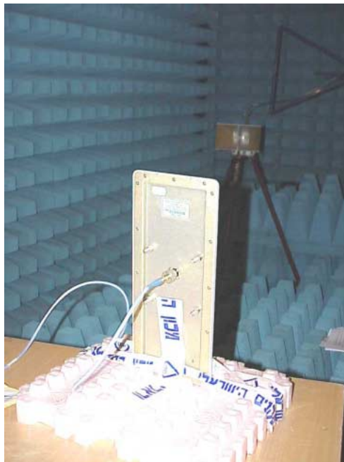
Photo # 5. P/N AN1152 Spurious emission test
