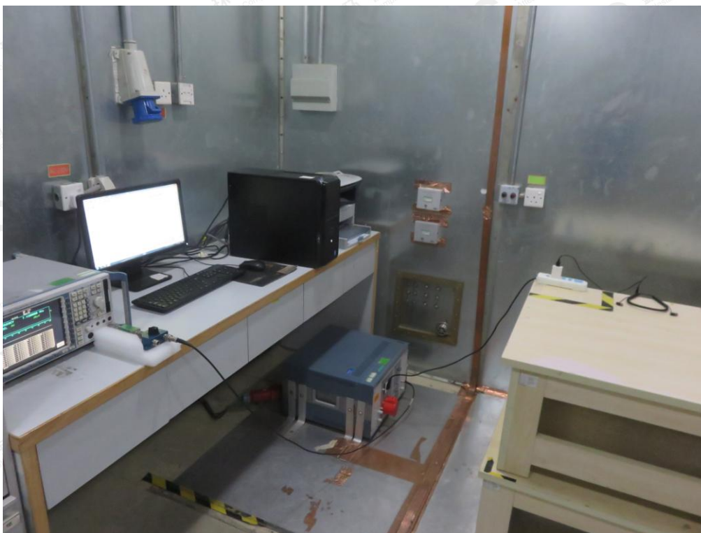
FCC RADIATED EMISSION TEST SETUP
