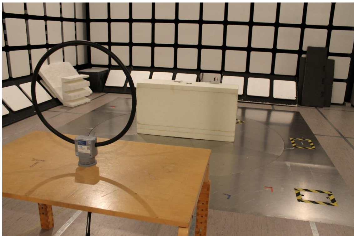
Photograph 2. Radiated Spurious Emissions 9 kHz - 30 MHz
