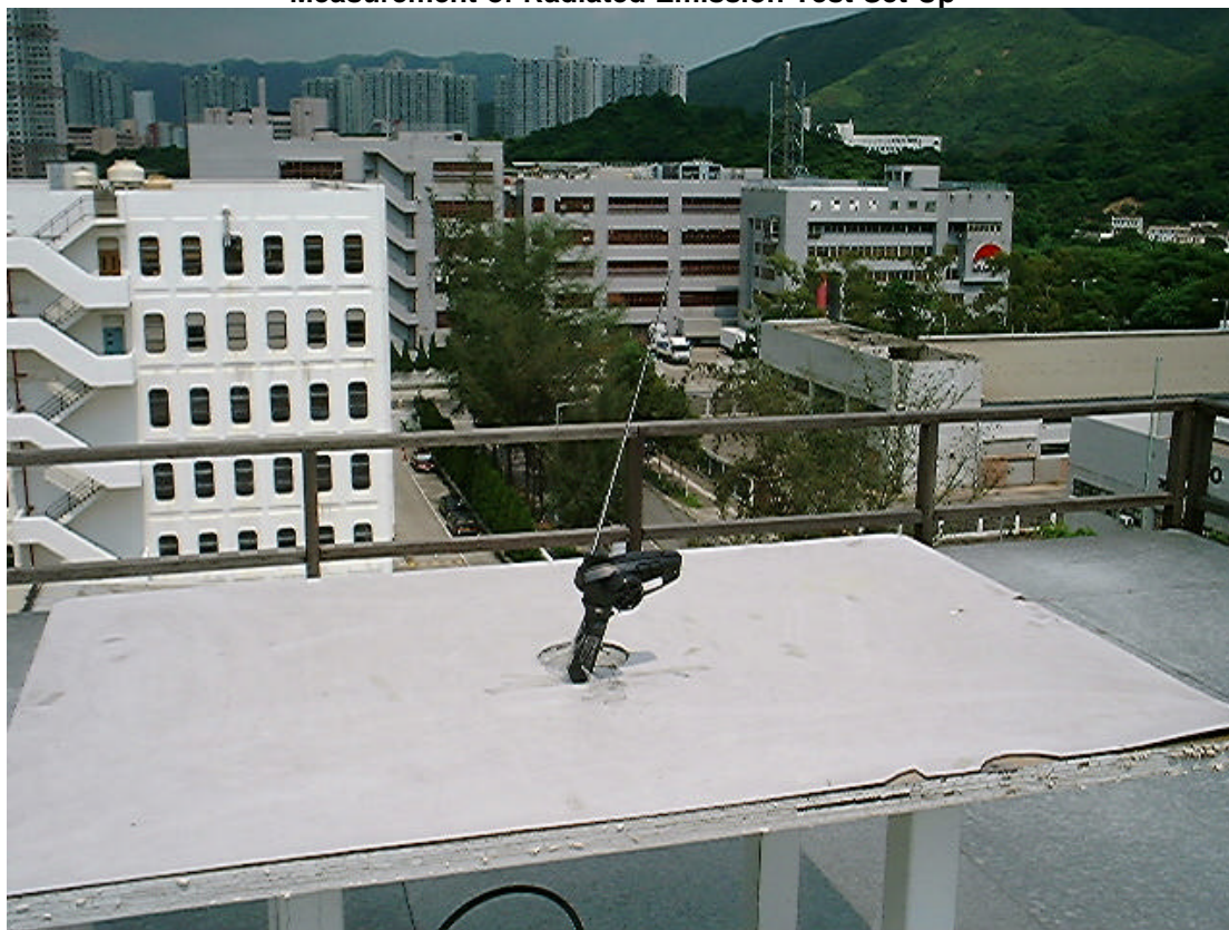
Measurement of Radiated Emission Test Set Up
