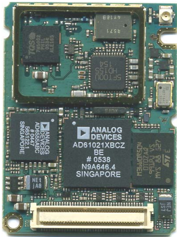
MC75: component side shielding opened
