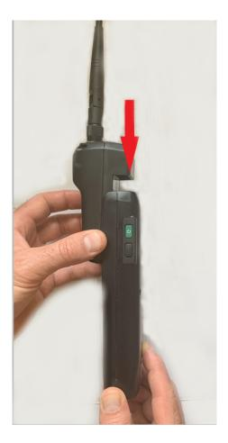
The screws on the Empower module will align with the screw holes on the EDB10.
