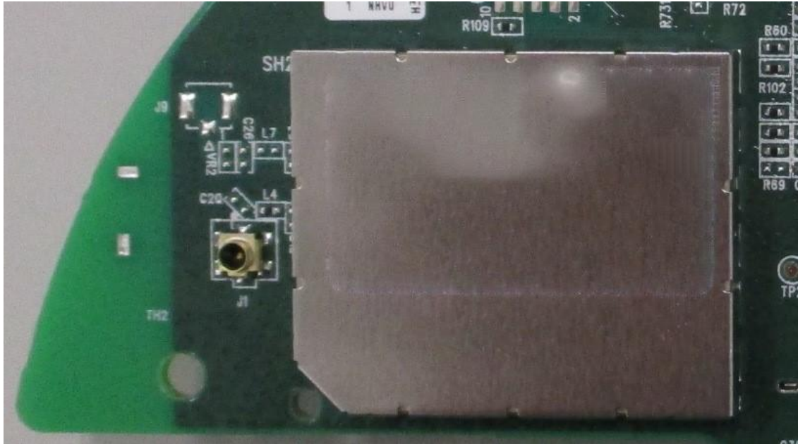
Connector for ZigBee conducted test
