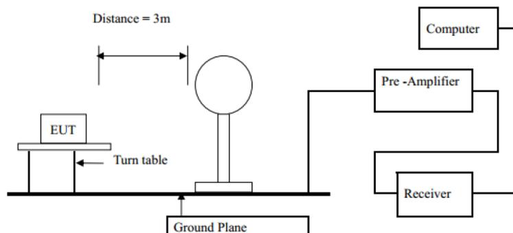
In 3m Anechoic Chamber Test Setup Diagram for frequency 30MHz-1GHz
