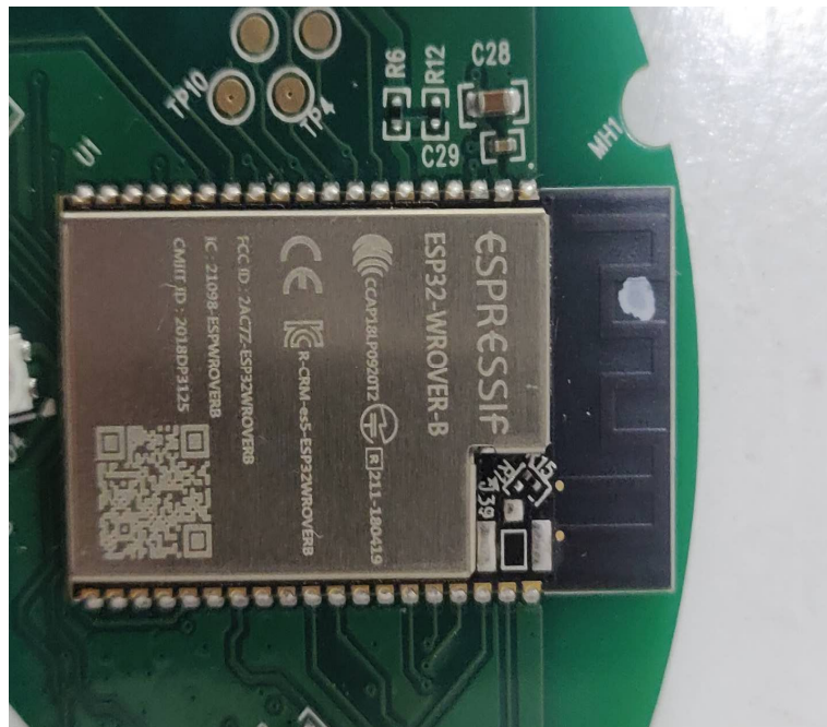
EUT –Wi-Fi Module Shielding View
