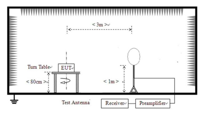
2) For radiated emissions from 30MHz to1GHz
