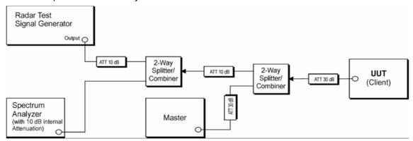
(Example Conducted Setup where UUT is a Client and Radar Test Waveforms are injected into the Client)
