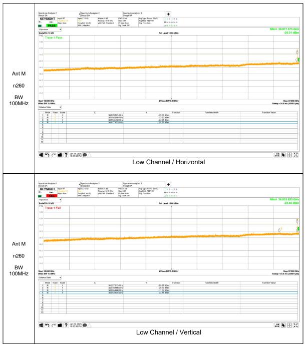
Note. If the margin of the pre-scan result is less than 3dB, the final measurement is performed for the identified spurious emissions.
