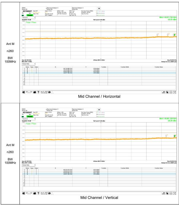
Note. If the margin of the pre-scan result is less than 3dB, the final measurement is performed for the identified spurious emissions.
