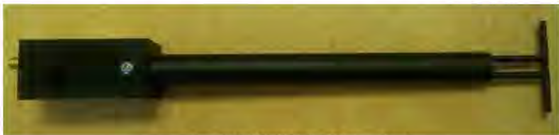
Figure 1 – MVG COMOSAR Validation Dipole
