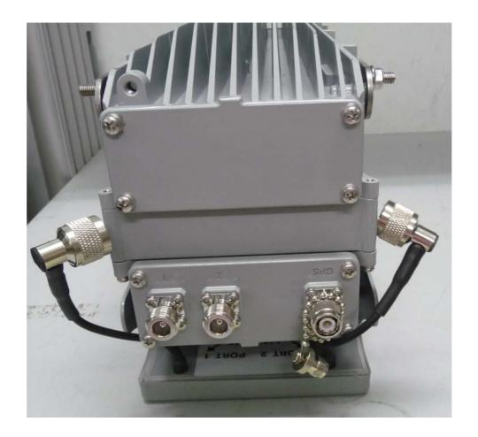
Photograph No.2 "AirHarmony 1000 2.5 GHz (B38, B41)" base station top panel view
