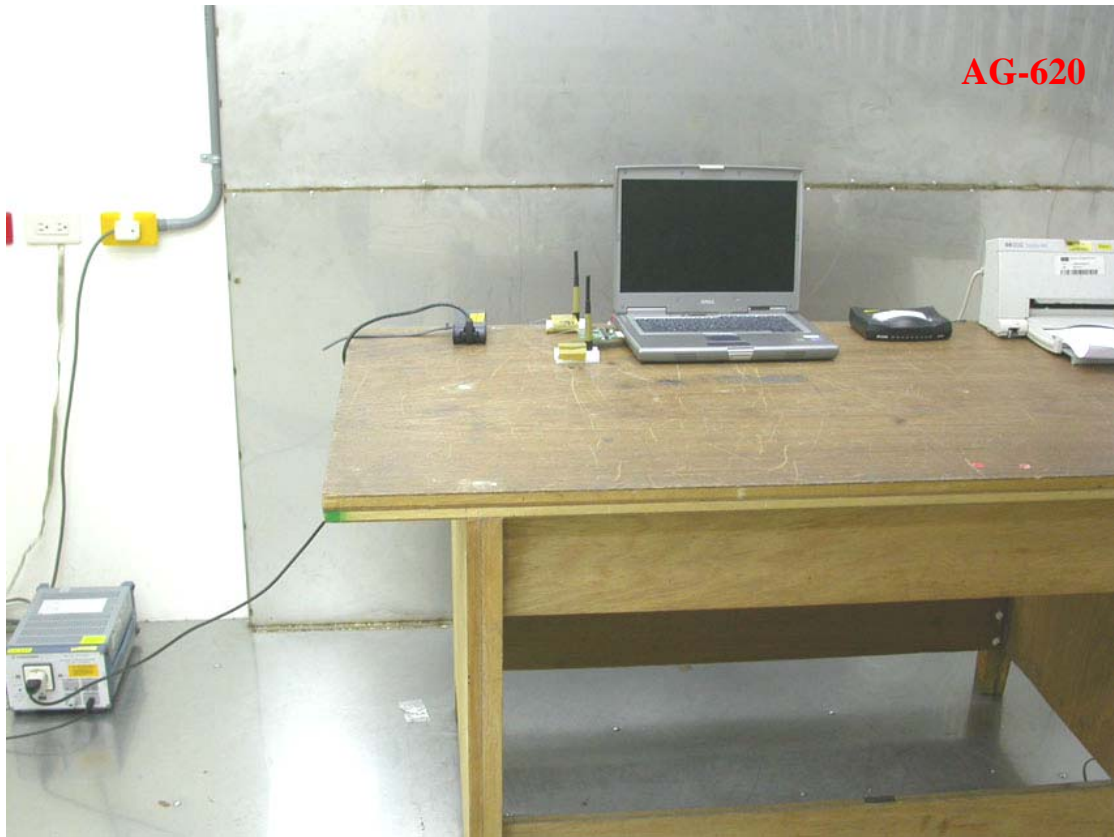
Photo 1: Conducted Emission Test Set-up photo
