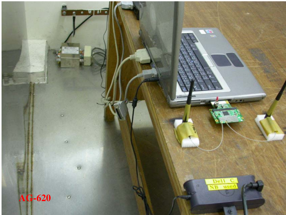
Photo 3: Conducted Emission Test Set-up photo
