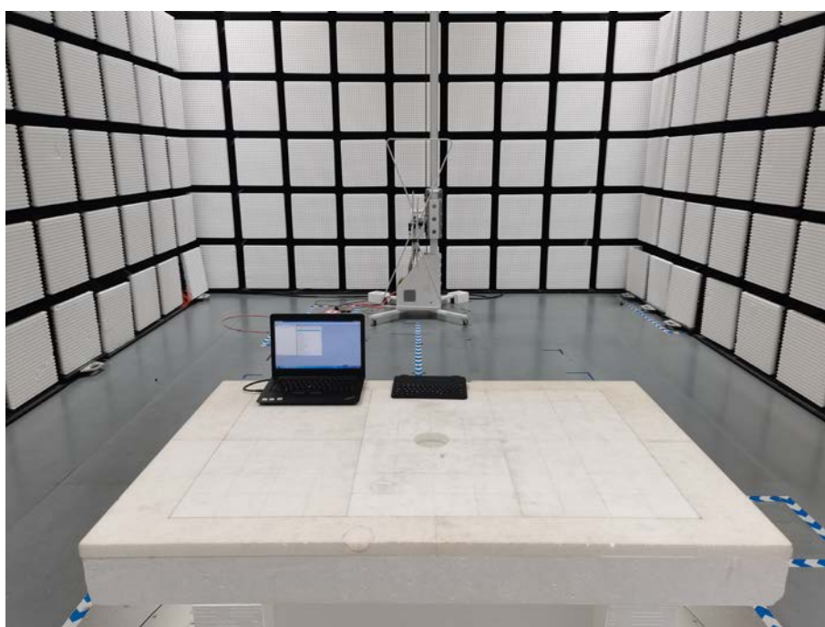
Fig. 2 Radiated emission setup photo(30MHz-1GHz)
