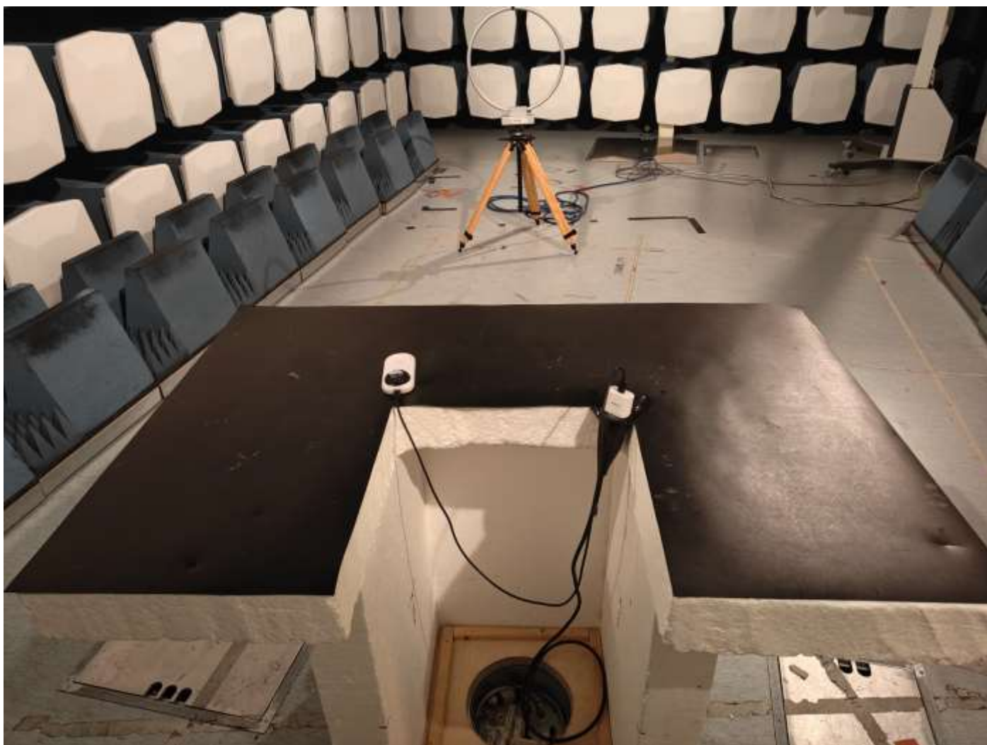
Picture 8 Radiated emission, view from EUT, 9 kHz -30 MHz
