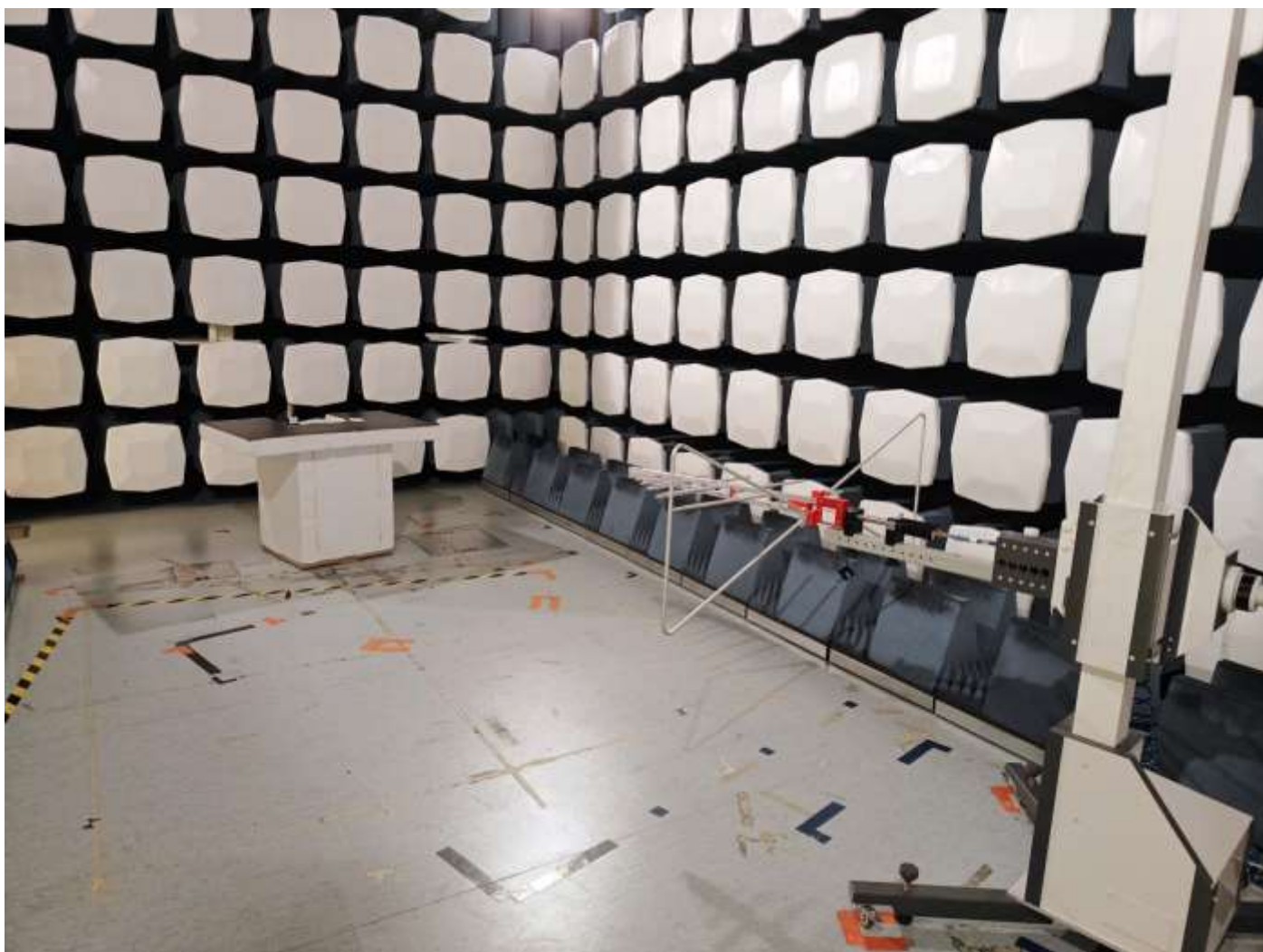
Picture 11 Radiated emission pictures, view from antenna, 30 – 1000 MHz
