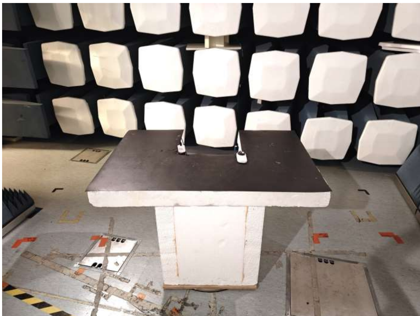
Picture 7 Radiated emission, common setup 9 kHz -1000 MHz
