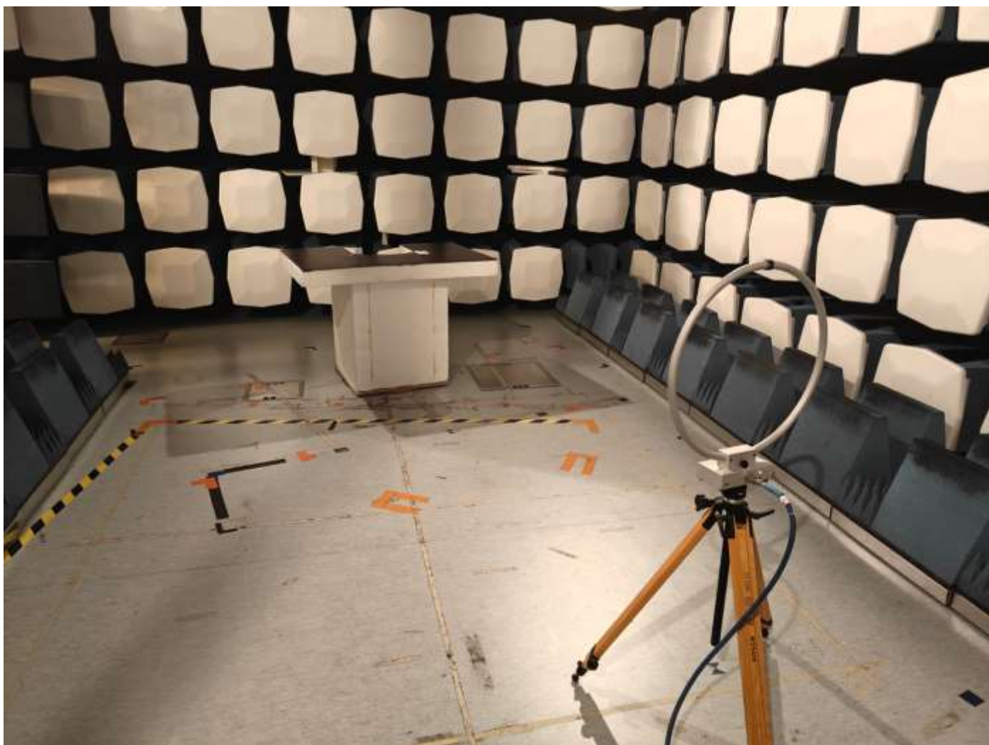
Picture 9 Radiated emission, view from antenna, 9 kHz -30 MHz
