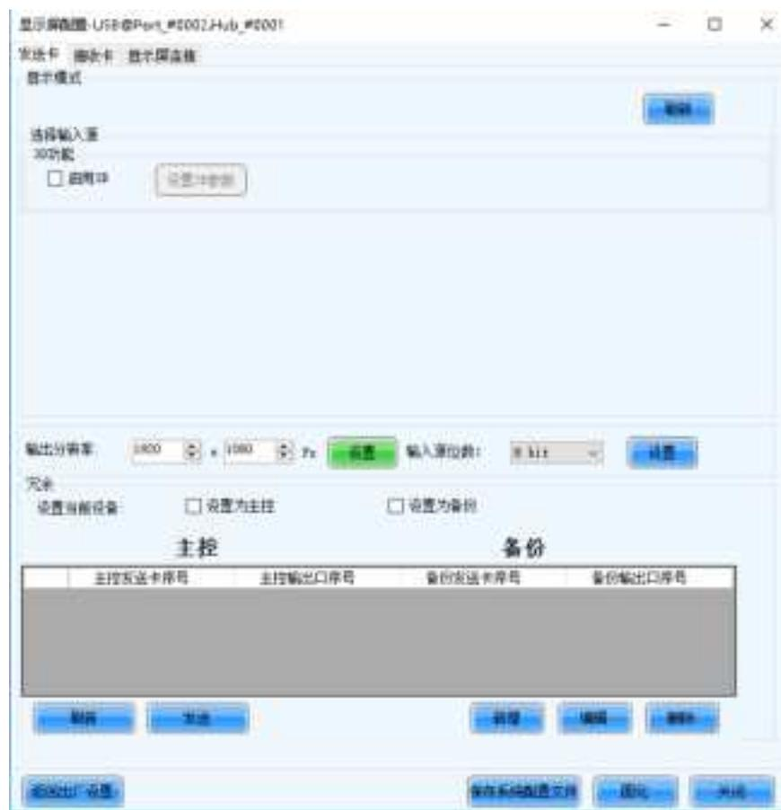
Step 4 Select the display screen connection, complete the M apping of the screen body according to the arrangement of the LED box and the signal routing, click to send it to the hardware and cure it for storage.
