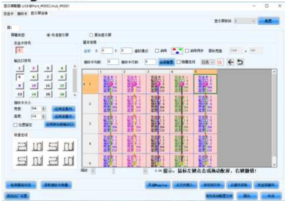
Note: The output port serial number is the output network port number on the control box, and the size of the receiving card is the display resolution of a single LED box.
