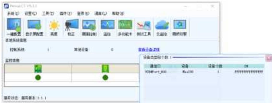
Step 3 Set the output resolution of the control box sending card. The output resolution is set to the resolution of the display screen. After clicking the set, solidify and save
