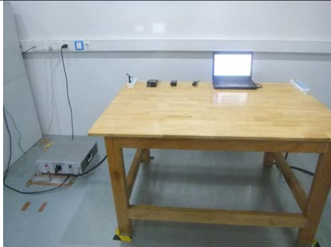
Conducted Emissions Test Setup Front View
