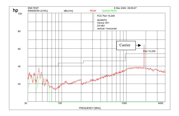
Carrier suppressed with a band rejection filter
