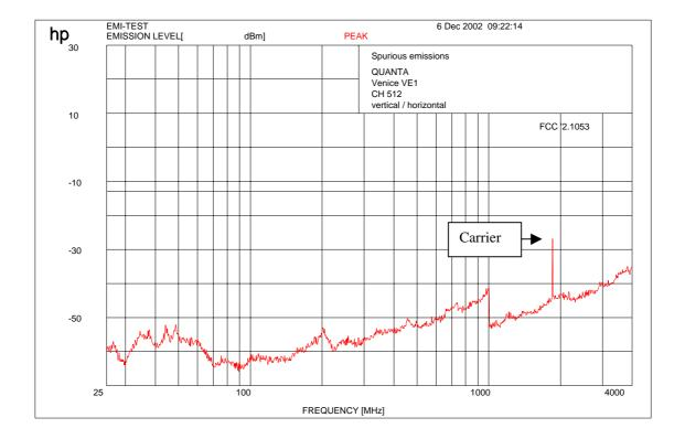
Carrier suppressed with a band rejection filter
