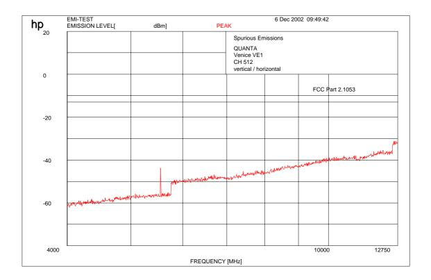
Carrier suppressed with a band rejection filter
