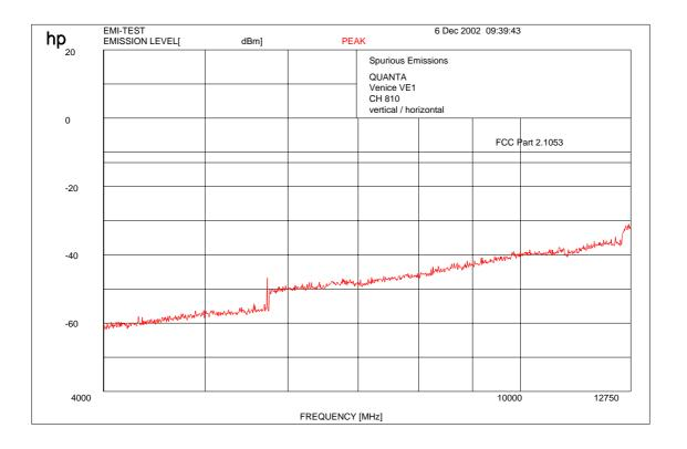
Carrier suppressed with a band rejection filter
