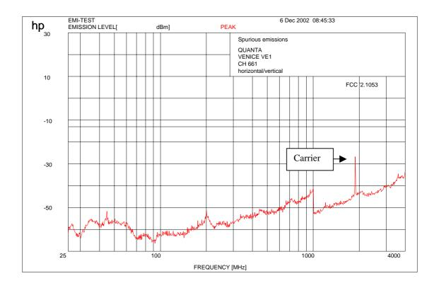
Carrier suppressed with a band rejection filter
