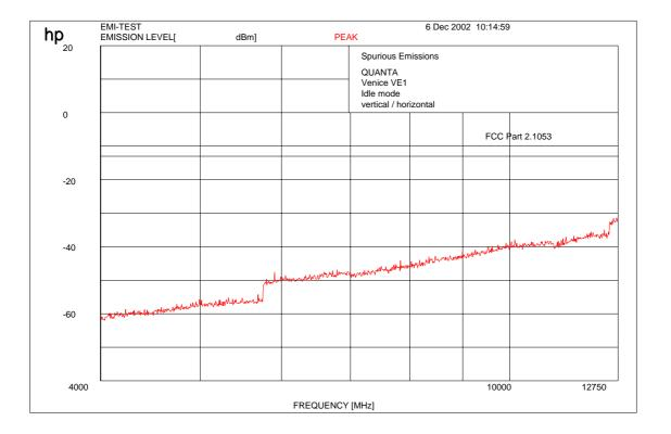
f < 1 GHz: RBW/VBW: 100 kHz  $f \ge 1 \text{GHz}$ : RBW/VBW: 1 MHz (Peak)
