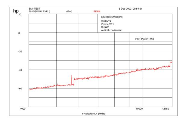
Carrier suppressed with a band rejection filter
