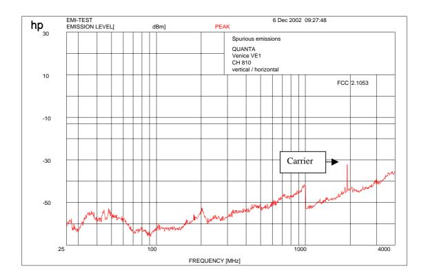
Carrier suppressed with a band rejection filter
