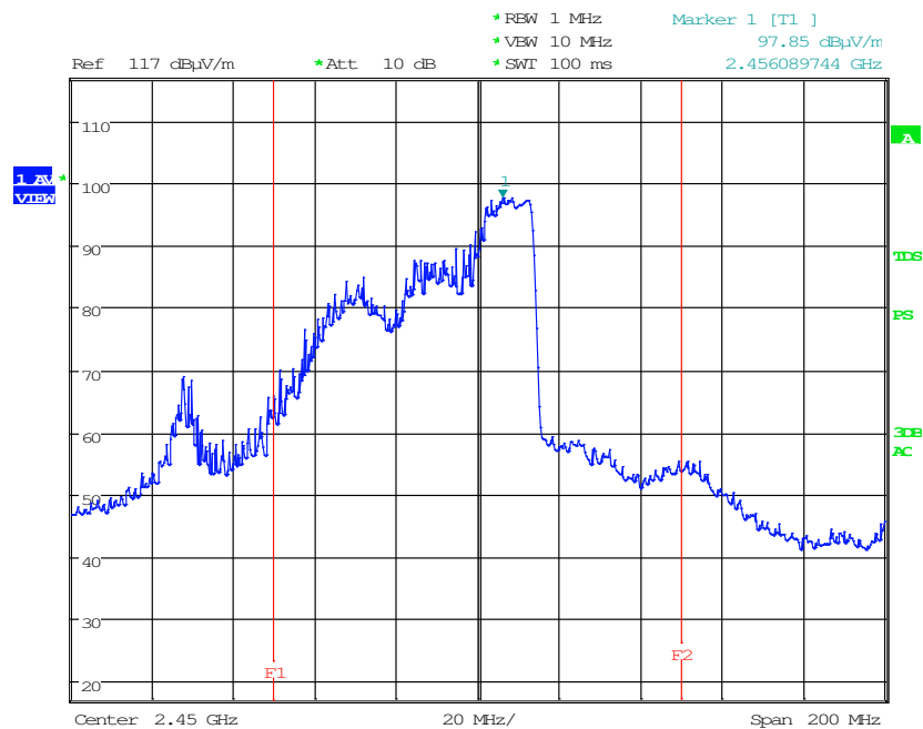
< Fig 8. Frequency Measurements (Minimum Frequency Observed: 2.456 GHz) >
