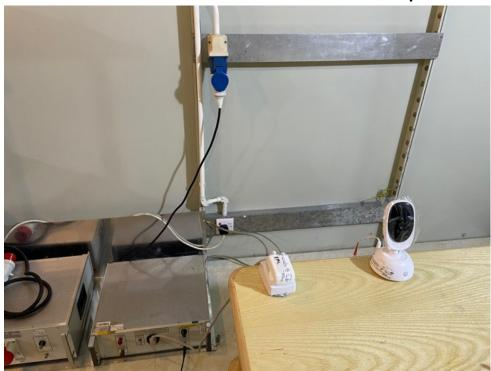
Radiated Emissions (30MHz-1GHz) Test Setup
