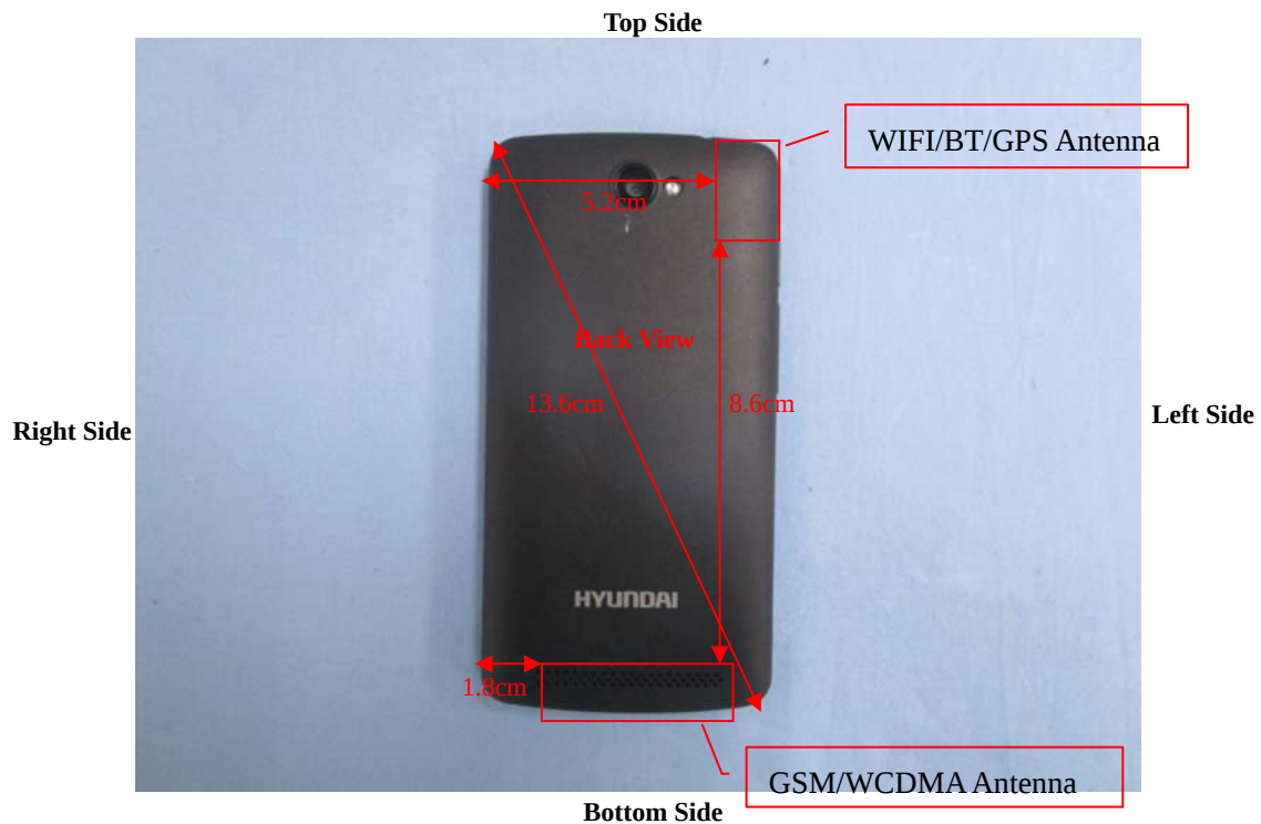
Block Diagram for EUT Antenna Position
