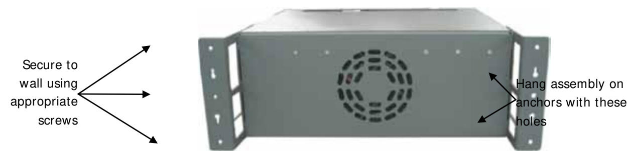
Figure 3-11. Bracket Mounted on Side of MA2000 TSX
