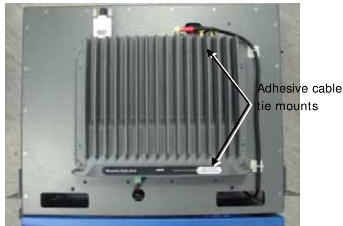
Figure 4-11. Secured High-Band connection
