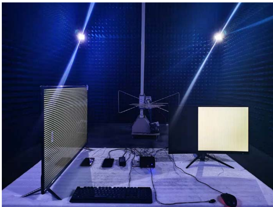
Photo of Radiated Emission Measurement (Below 1G)
