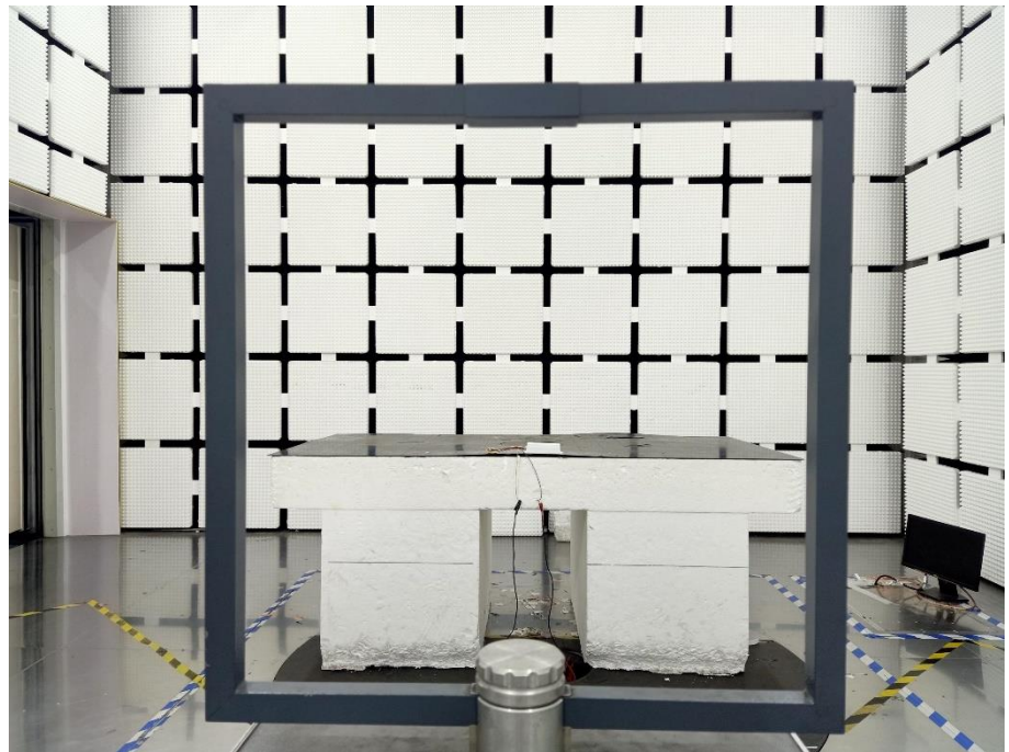
Radiation Emission Test Setup (Below 30MHz)
