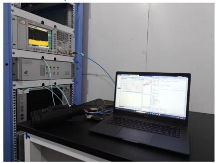
Conducted Emissions at AC Power Line (150kHz-30MHz)
