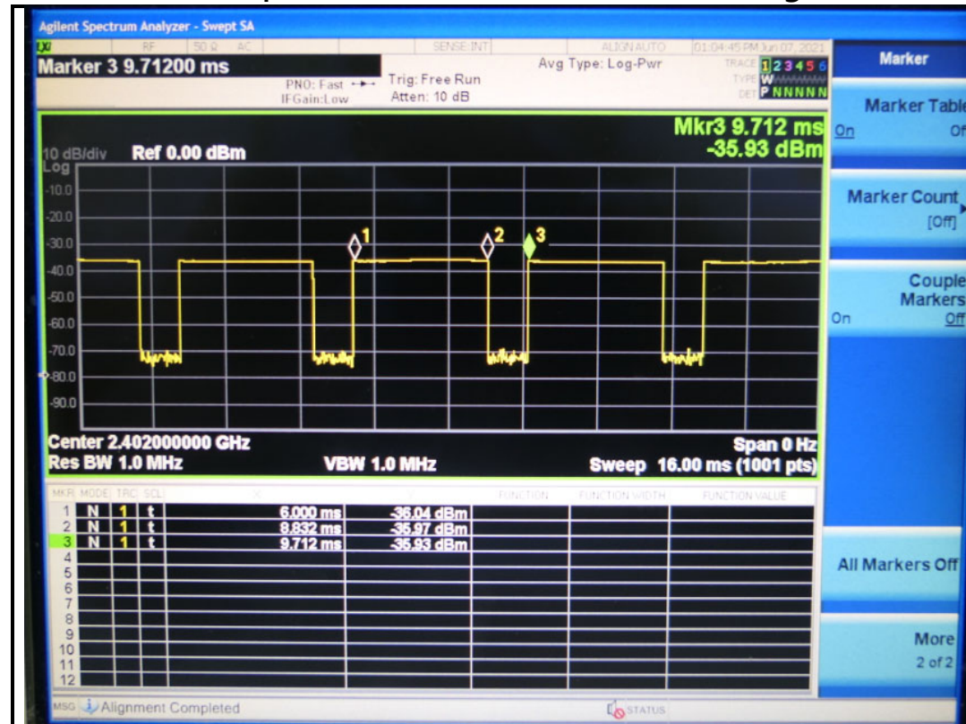
Time-domain plot for Bluetooth transmission signal
