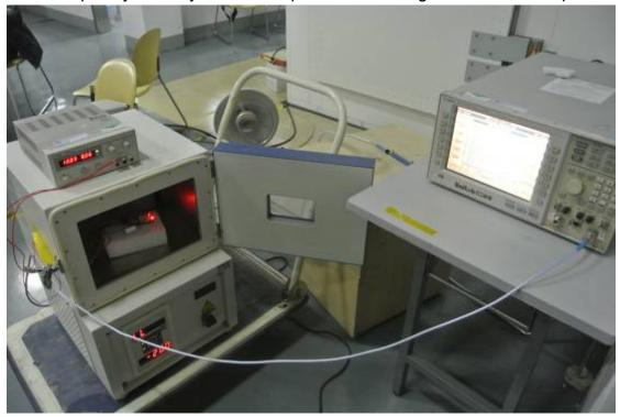
Radiated Spurious Measurement(below 30MHz) Setup
