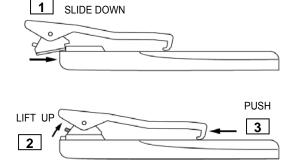
Gently slide the clip into the appropriate guides located in the transceiver's back until it firmly locks.
