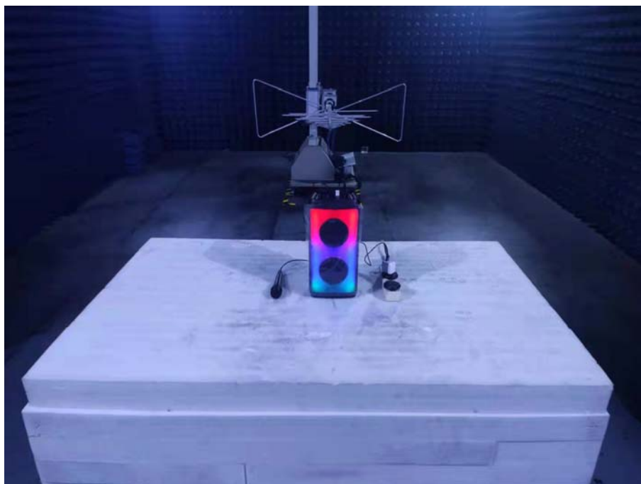
Photo of Radiated Emission Measurement Below 1GHz
