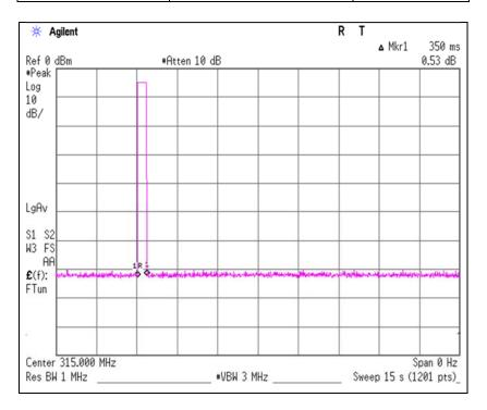
\* The EUT transmits UHF when LF signal is received from a car or a button on the EUT is pressed. In both cases, the UHF transmission is stopped within 5 seconds. So the test was performed by a button-pressed operation as the worst case.
