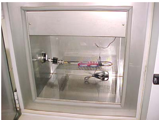
The Temperature Chamber
