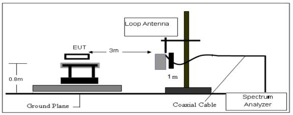
(B) Radiated Emission Test-Up Frequency 30MHz~1GHz
