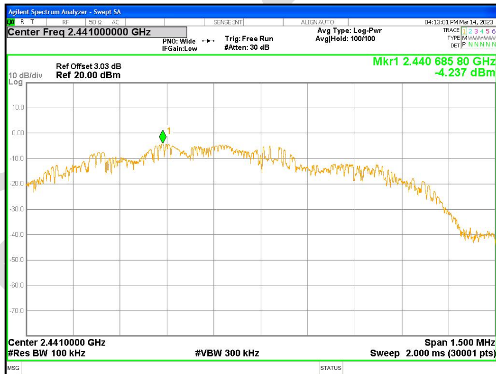
Tx. Spurious NVNT 2-DH1 2441MHz Ant1 Emission
