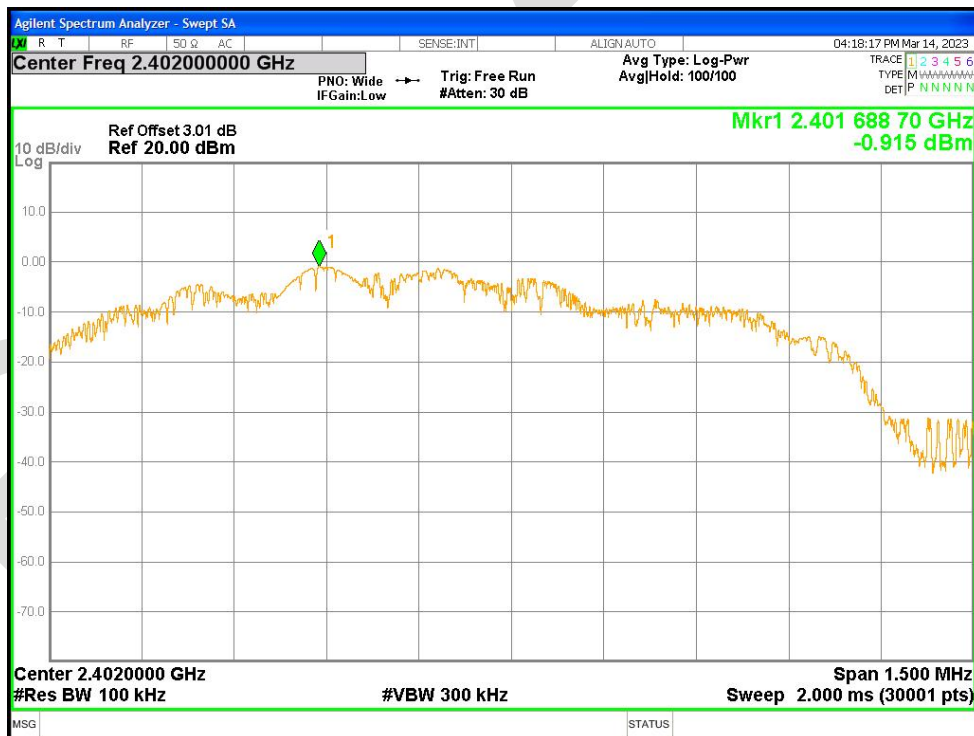
Tx. Spurious NVNT 3-DH1 2402MHz Ant1 Emission
