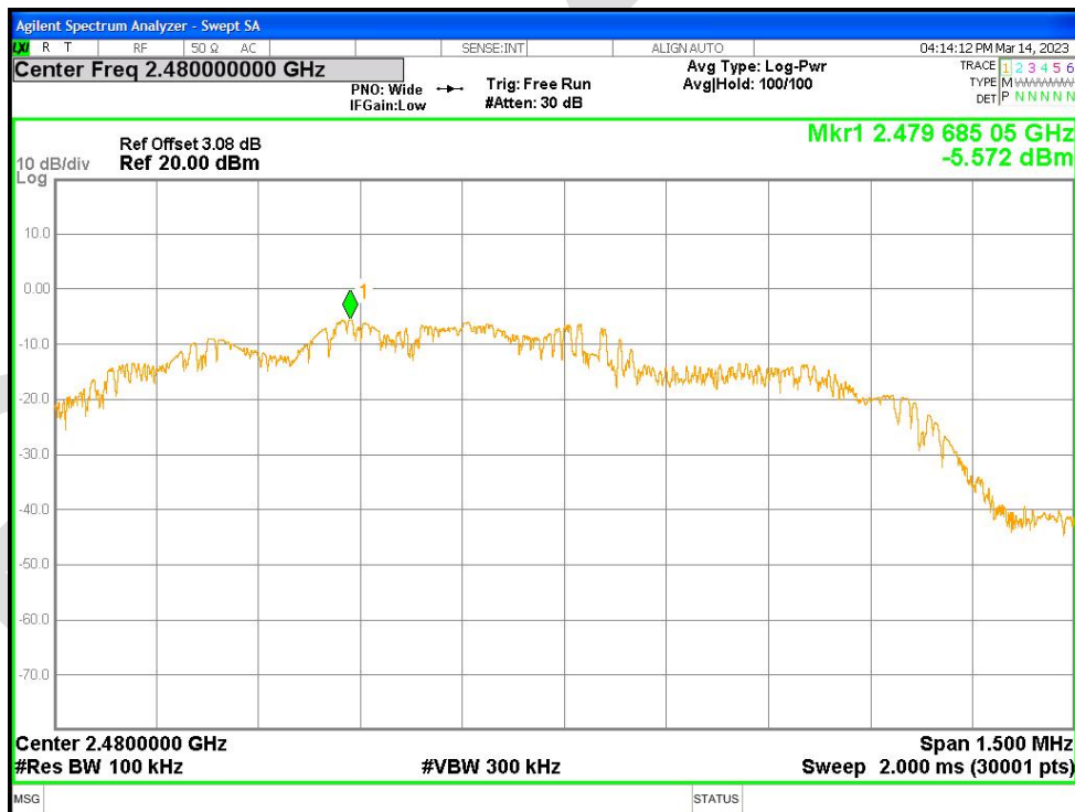
Tx. Spurious NVNT 2-DH1 2480MHz Ant1 Emission
