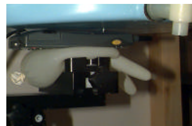
Figure 18. Hand SAR Test Setup
