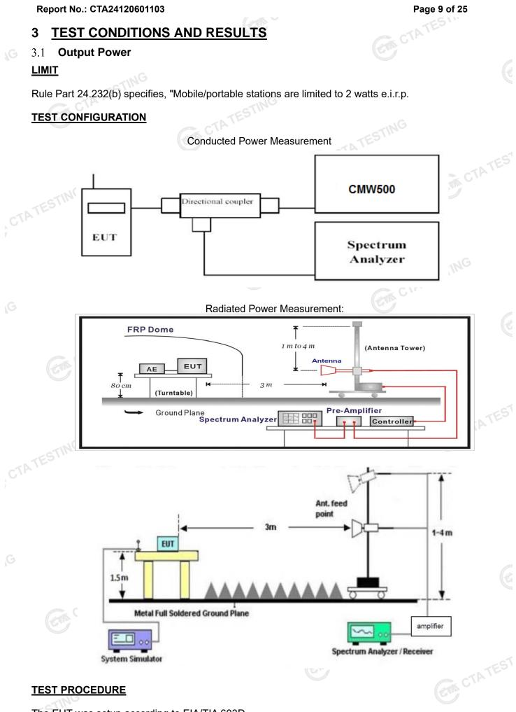
The EUT was setup according to EIA/TIA 603D
