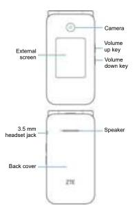
Setting Up Your Phone Power off your phone before installing or removing the nano-SIM card, the microSDHC card (optional), or the battery.
