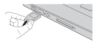
The first time you plug a USB device into a particular USB port on your computer, Windows automatically installs a driver for that device. After the driver has been installed, you can disconnect and reconnect the device without performing any additional steps.
