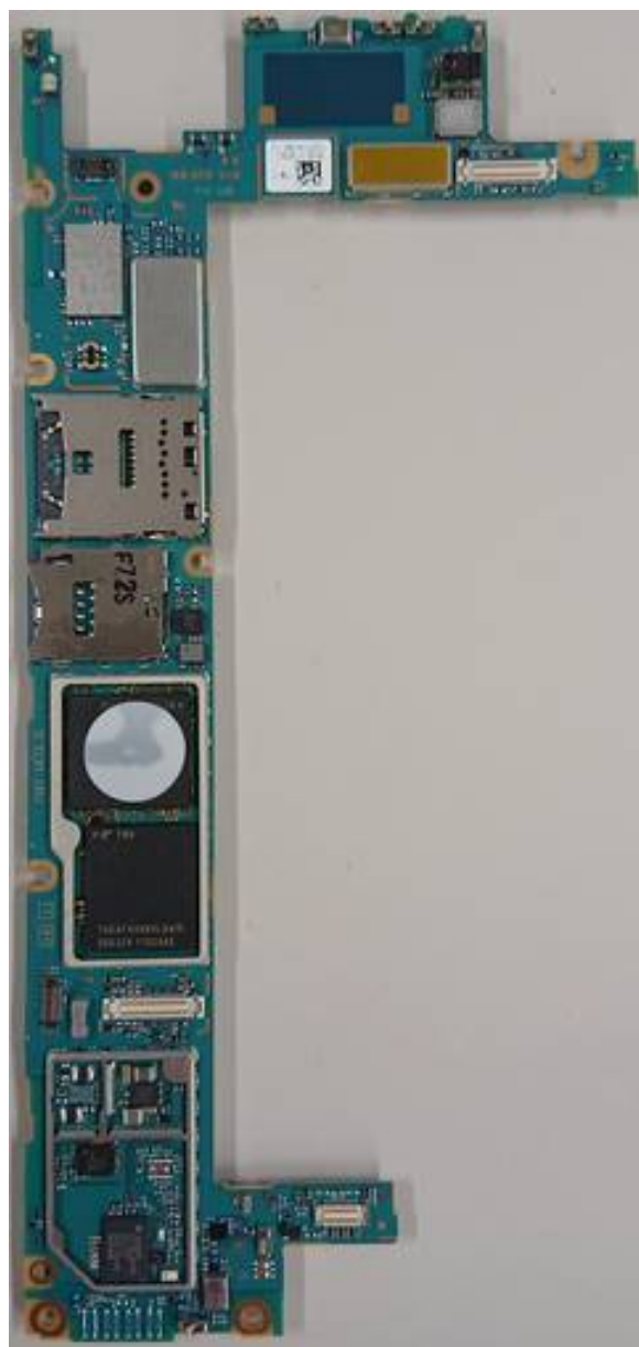
Internal PWB without Shield cases (Front-side)
