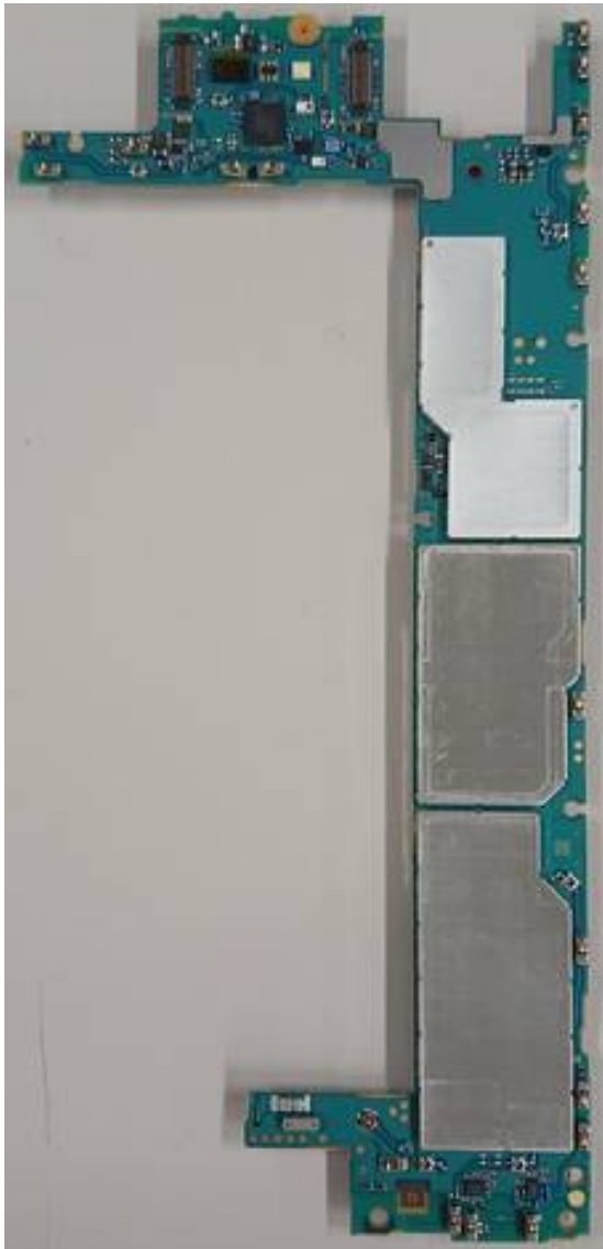
Internal PWB with Shield cases (Rear-side)
