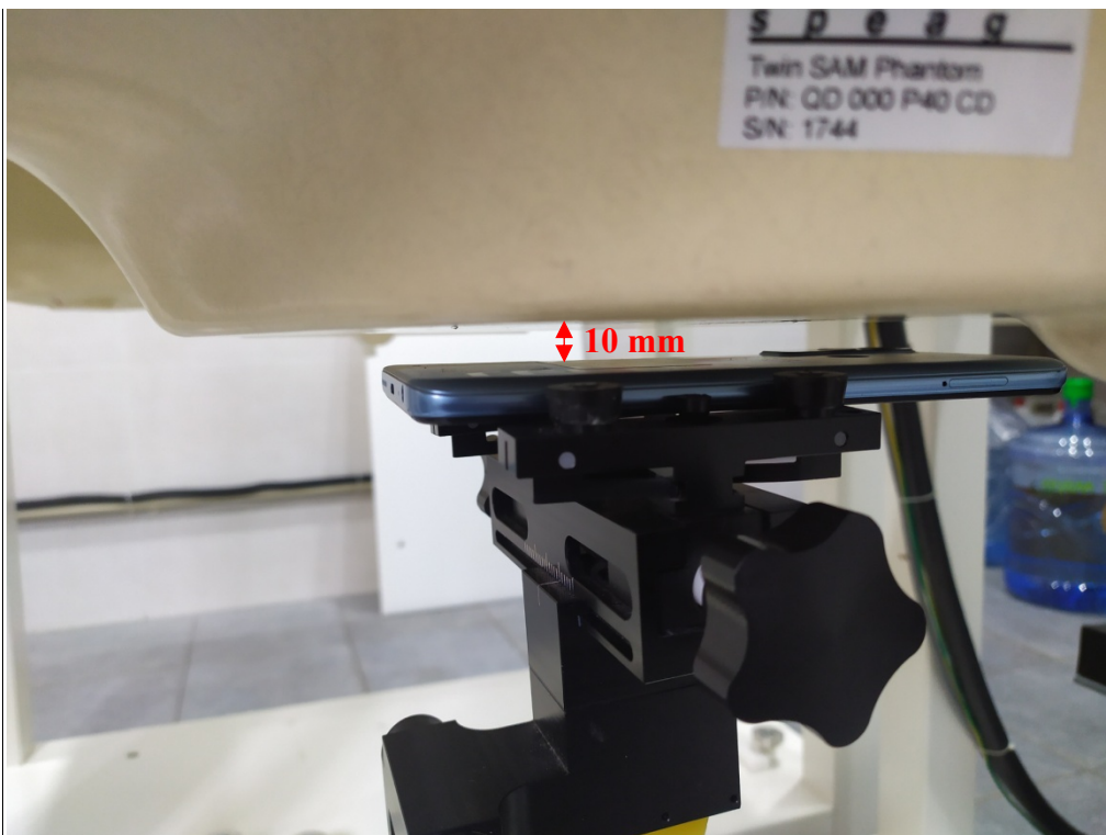
Body (Worn) Back Setup Photo (10mm)
