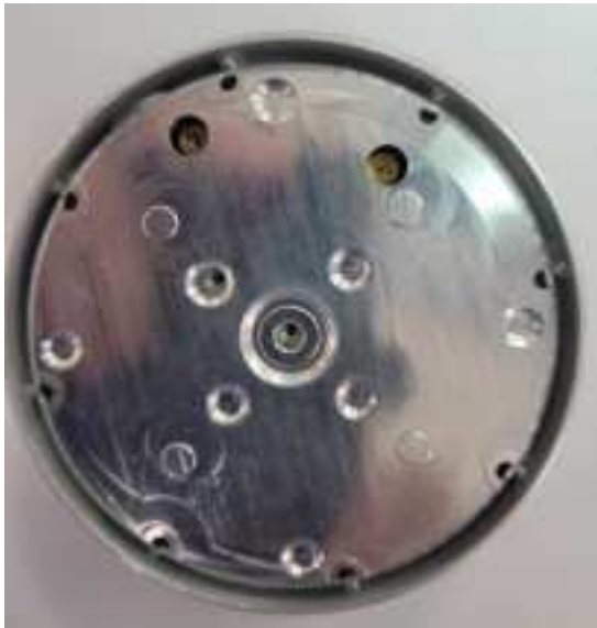
Yahsat T-TAC Maritime Antenna Step 3 – Mounting of Inner Shield
