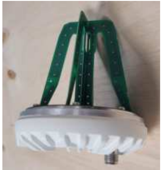
Yahsat T-TAC Maritime Antenna Step 4 – Mounting of Antenna Module
