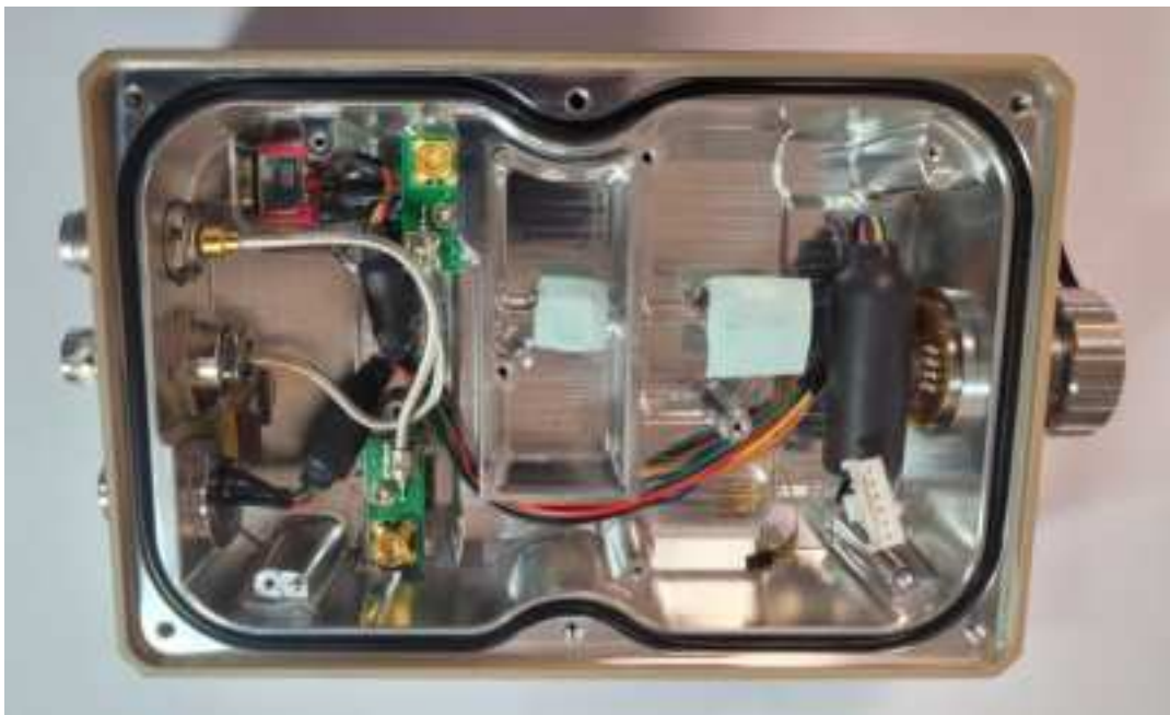
408060A Yahsat T-TAC GCU without PCBA and Lid.
