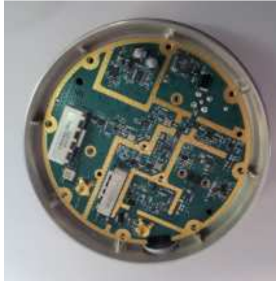
Yahsat T-TAC Maritime Antenna Step 2 – Mounting of PCBA
