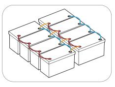
Connect the paralleled battery systems in series.
