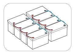
Connect the batteries in parallel.
