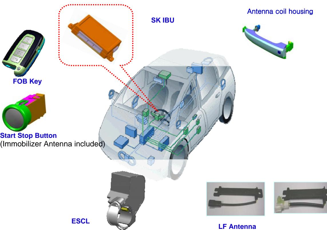
**Figure 1: Offered System Components**
