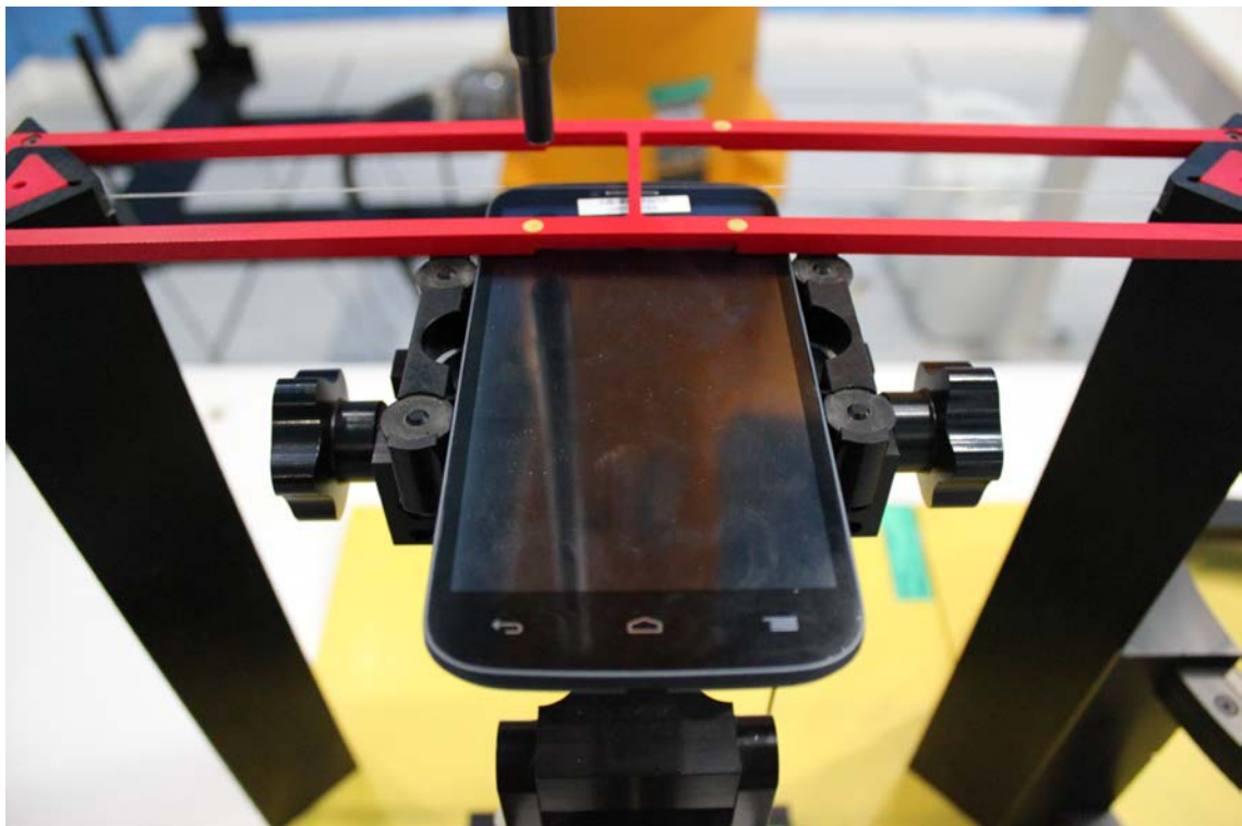
Picture 2: EUT Positioning for RF
